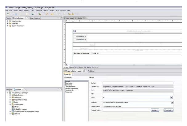
Set any parameter display fields. Do not drag parameters from the Data Explorer into the report. Instead, drag a Data element and set the Value Expression to the parameter.
