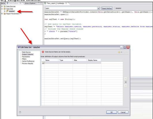
Set the data type for each output column based on the maxtype of the field. The chart below shows the Maximo Database Type, the corresponding BIRT Data Type, and the method used within the BIRT Designer to retrieve its value.
